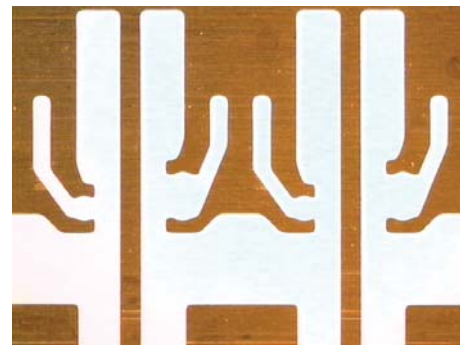
Figure 3: Lead frame configuration for an 0402 and 0603 fuse.
